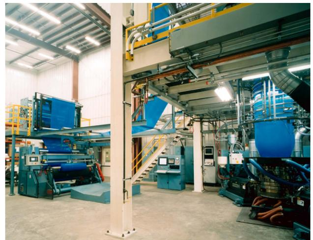
*Davis Standard maintains a complete production system for in-house development and customer demonstrations, including blown film (right) and film winding (left).*
