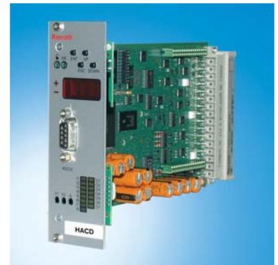
*The VT-HACD digital hydraulic axis controller offers sophisticated control in a compact format.*
