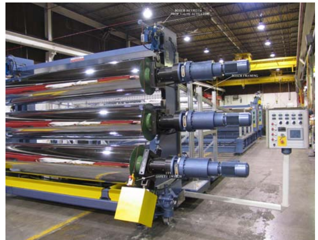
Welex takeoff machine offers superior roll-gap control using a hydraulic system from Bosch Rexroth.
